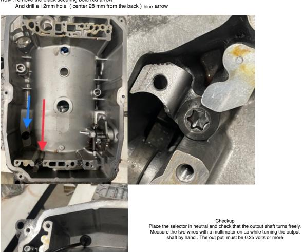
Measure the two wires with a multimeter on ac while turning the output shaft by hand . The out put must be 0.25 volts or more
